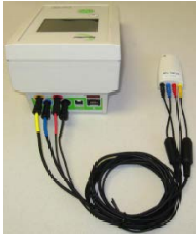
Figure 3.1 Impedimed Multifrequency Analyzer (IMA) (Model SFB7) with Test Cell. [52]
