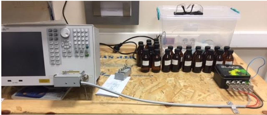
Figure 3.2 Impedance Analyzer and shielded electrode measurement box.
