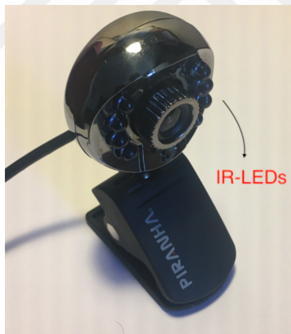
Figure 2.13 Webcam with IR-LEDs that is used to capture eye blinks.
