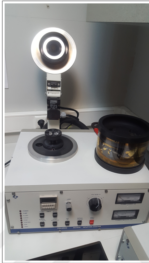
Figure 2.10 Platinum sputtering before SEM.
