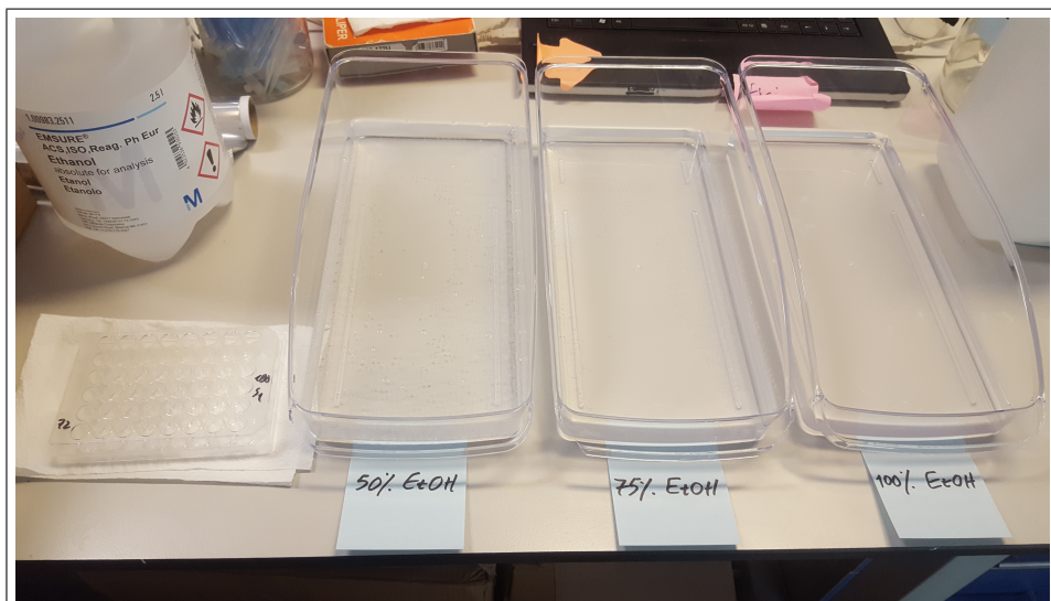
Figure 2.8 Sample dehydration by successive immersion in ethanol.
