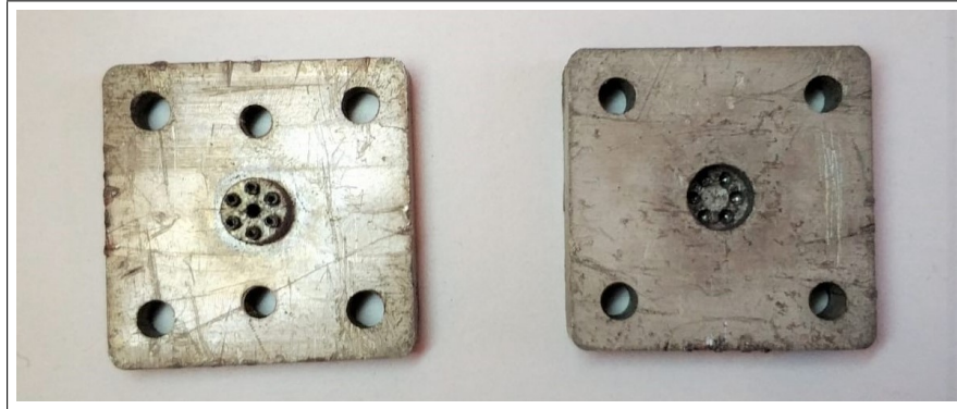
Figure 3.22 The aluminum mold used for shape setting procedure of distal anchor structure.
