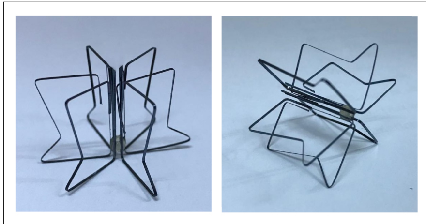
Figure 3.20 Occluder frame with curved end flat nitinol wires.
