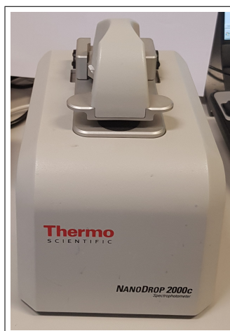
Figure 3.1 NanoDrop 2000c Spectrophotometer (Thermo Scientific, Barrington, IL, USA) was used to measure the absorbance spectrum to test the photoactivity of 10 \mu\text{M} Curcumin.
