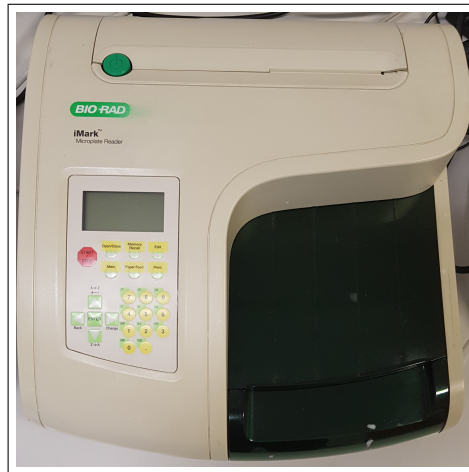
Figure 3.6 iMark microplate reader (Bio-Rad Labs, Sunnyvale, CA) was used to measure the optical density.
