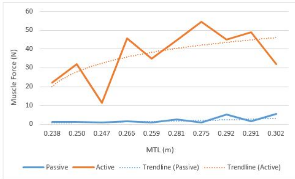
Figure 3.12 Limb 4 GRA muscle-tendon complex length vs. muscle passive and active forces.
