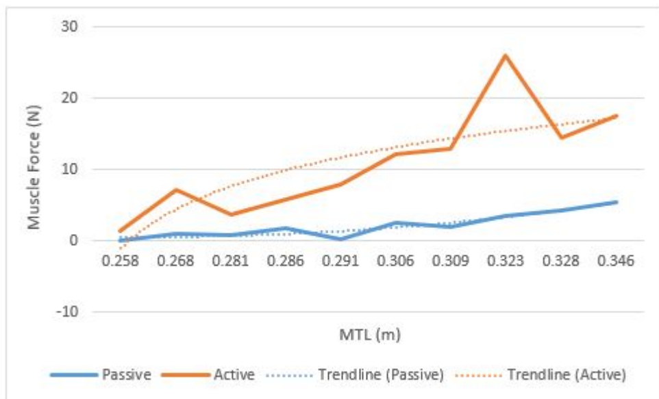
Figure 3.13 Limb 4 ST muscle-tendon complex length vs. muscle passive and active forces.
