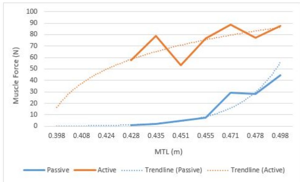
Figure 3.4 Limb 1 ST muscle-tendon complex length vs. muscle passive and active forces.
