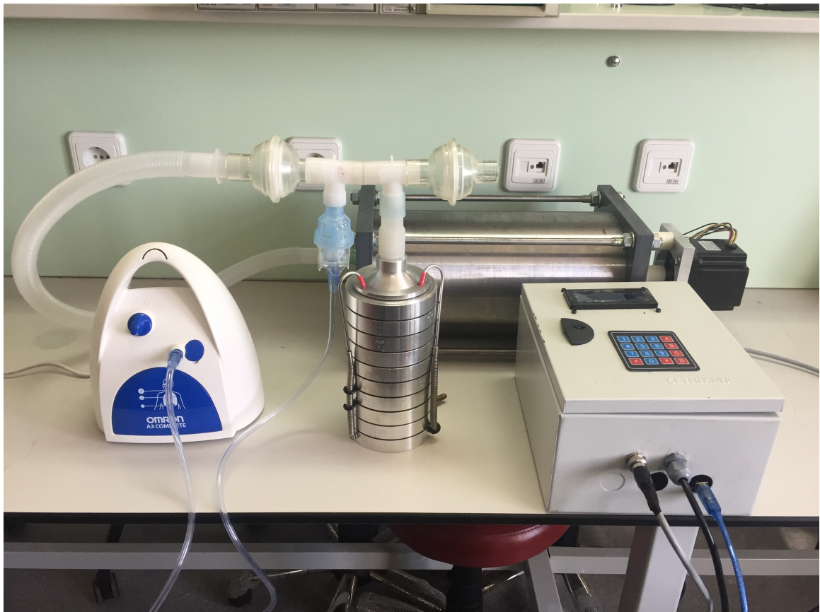
Figure 3.12 Test apparatus for testing the nebulizer output.
