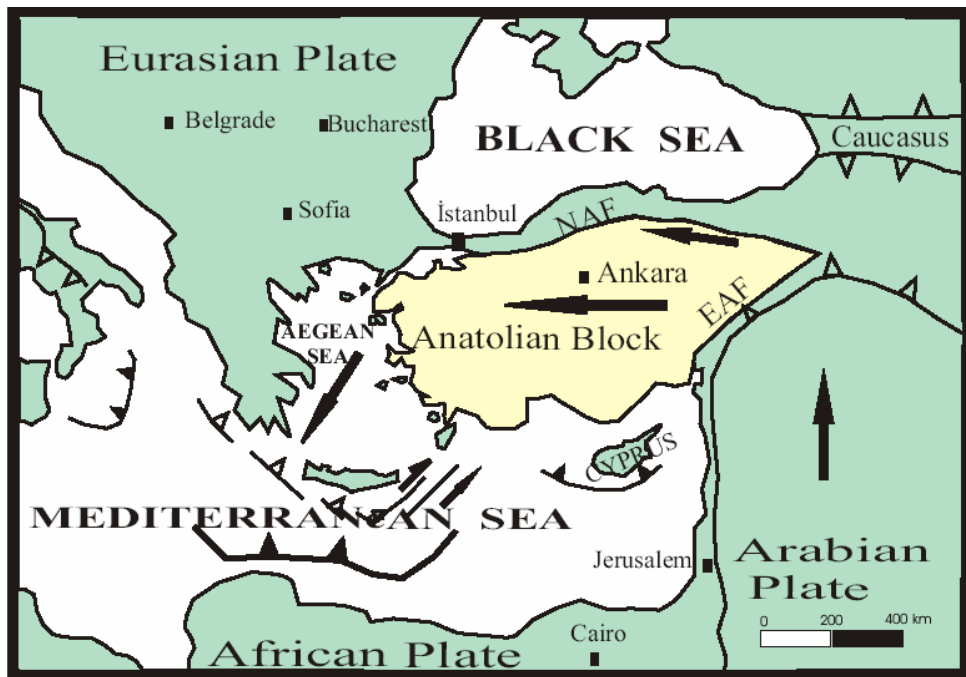
Figure 3.1. Map showing the plate motions which is effective on the tectonics of Turkey (Okay et al., 1999).
