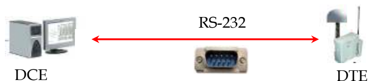
Figure 3.8. Direct serial connection between DTE and DCE
