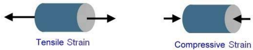
Figure 4.2. (a) Tensile strain (b) Compressive strain
