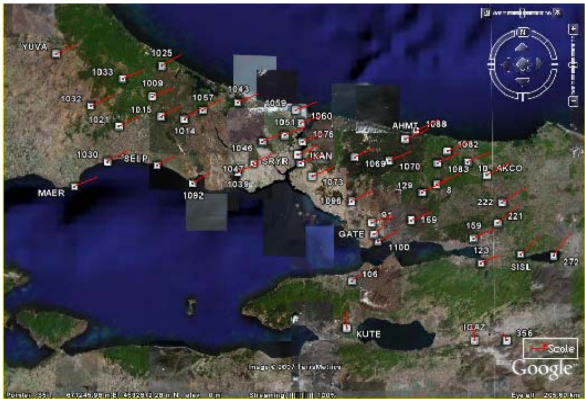
Figure 3.1. Displacement vectors between 2006.60 and 2000.45 epochs
