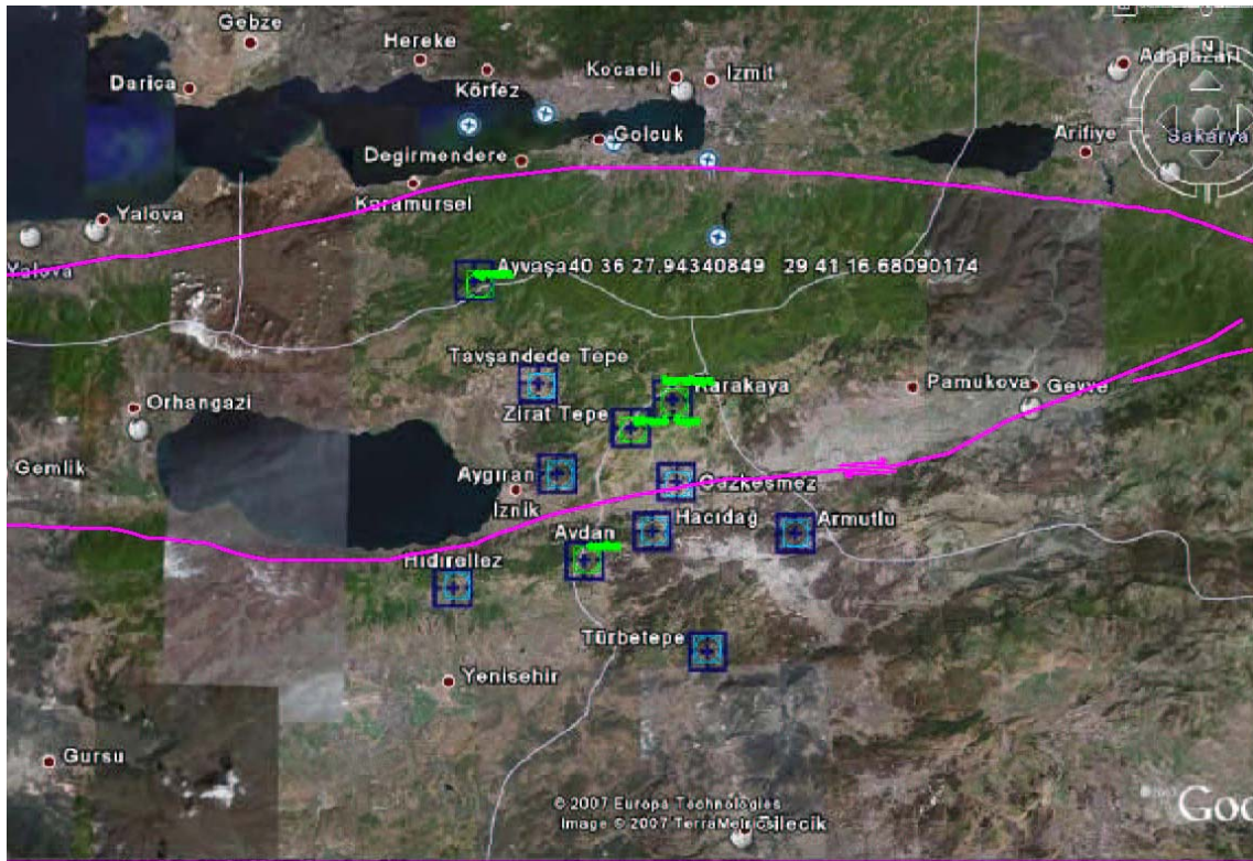
Figure 3.1. The constellation of GCM_ITU network. The green marks display the terrestrial stations which could not prevail for GPS campaigns.
