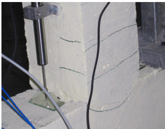
Figure 2.9. Measuring plastic rotations occurred in the system
