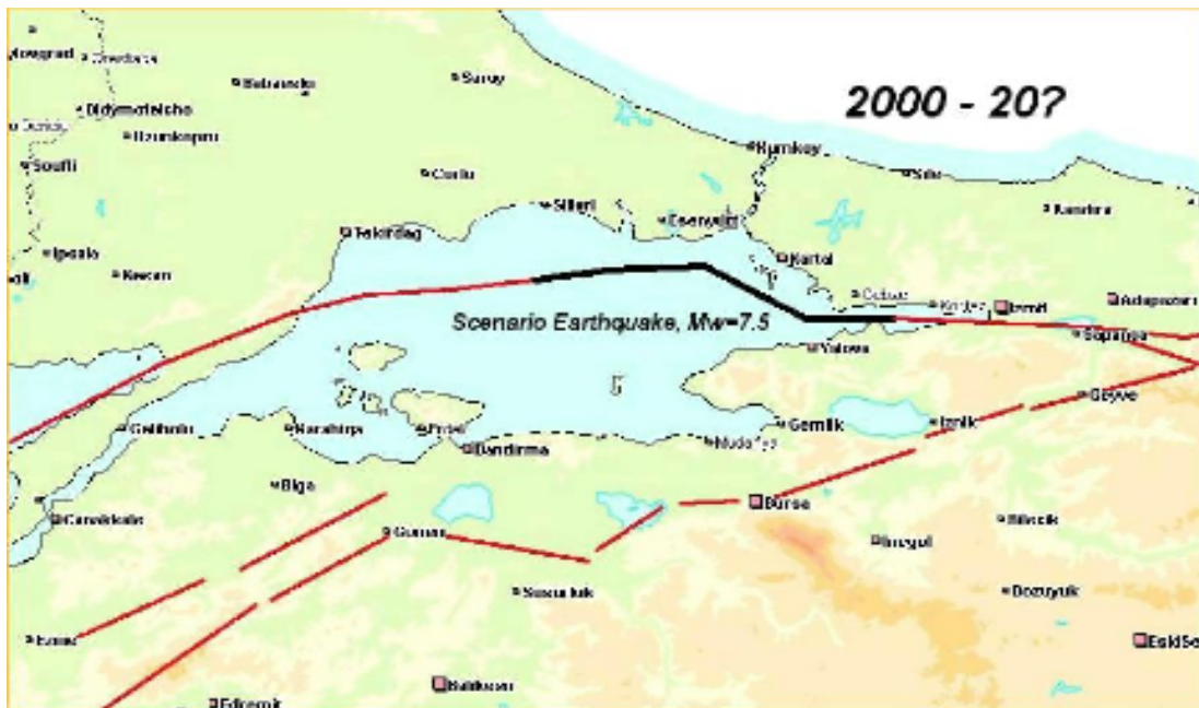
Figure 3.14 Mw=7.5 scenario earthquake for İstanbul and vicinity (Erdik et al. , 2002)
