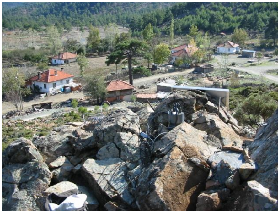
Figure 5.4. Installation of the seismometer at the station TURG on 15 December 2006
