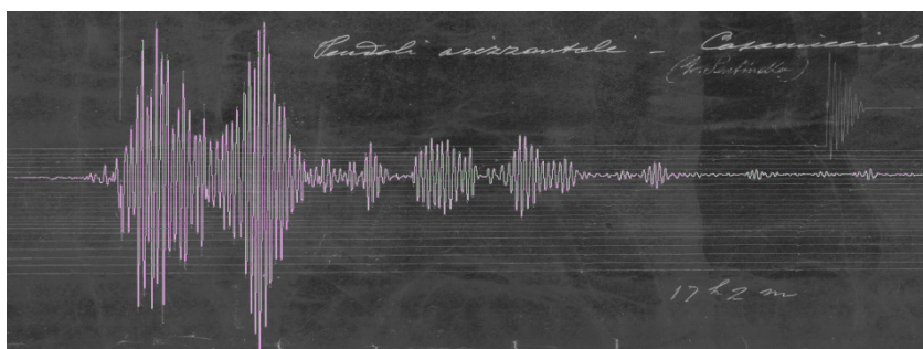
Figure A 2. Digitized seismic traces on original E-W seismogram of 08.09.1912, 01:29 Earthquake from IC1H station, recorded by Horizontal Pendulum
