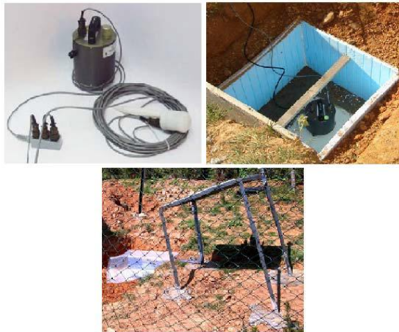
Figure 4.4. CMG-6TD with supplied GPS and installation site of a station.
