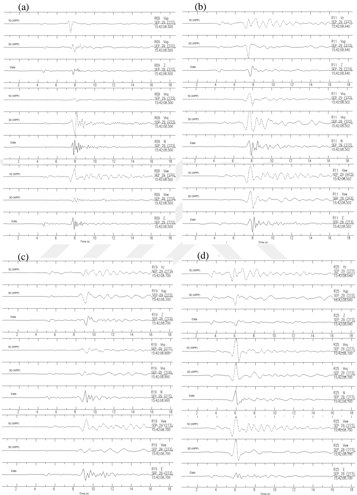
Figure 6.4. Comparison of three component 1D and 3D synthetics with real data for 29 September 2009 earthquake at stations R09 (a) located in Kadıköy, R11 (b) located in K.Bakkalköy, R19 (c) located in Fatih and R25 (d) located in Maltepe.
