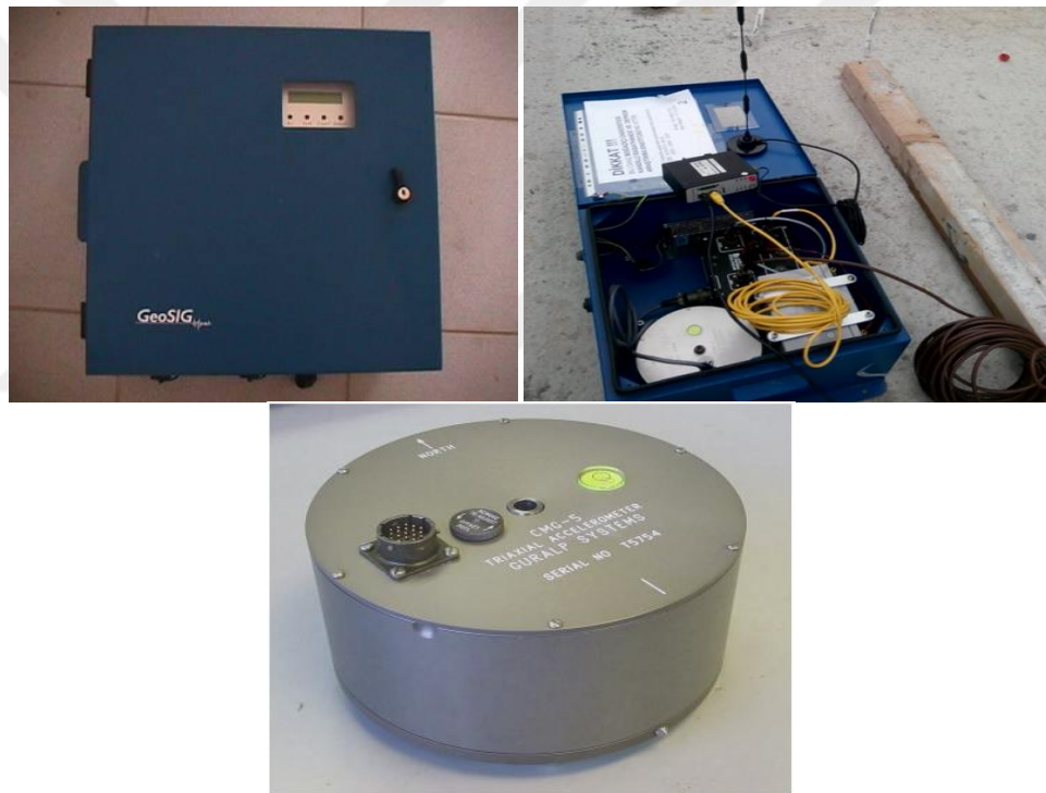
Figure 4.2. Strong motion accelerometer and transducer
