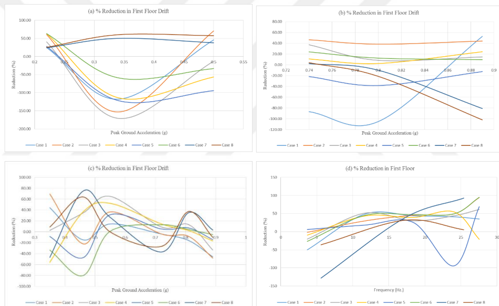
Figure 5.7. Reduction in First Floor Drift under (a) Kocaeli Earthquake, (b) Kobe Earthquake, (c) El Centro Earthquake, (d) Cyclic Sinusoidal Motion for GSI-CL.
