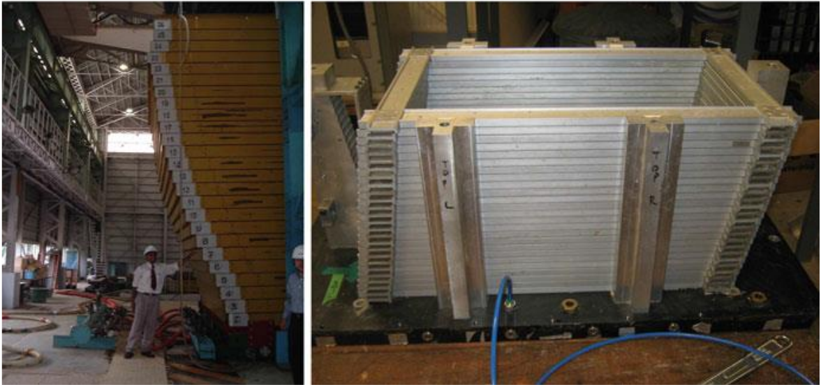
Figure 2.63. Examples of Laminar Containers (Prasad et al. , 2004; Bhattacharya et al. , 2012).
