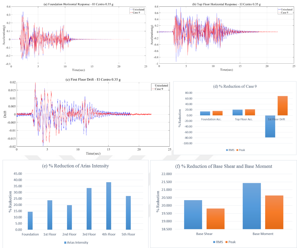
Figure 4.33. (a) Foundation Acceleration Response, (b) Top Floor Acceleration Response, (c) First Floor Drift Response, (d) % Reduction of Case 9, (e) % Reduction of Arias Intensity, (f) % Reduction of Base Shear and Base Moment under El Centro Earthquake.
