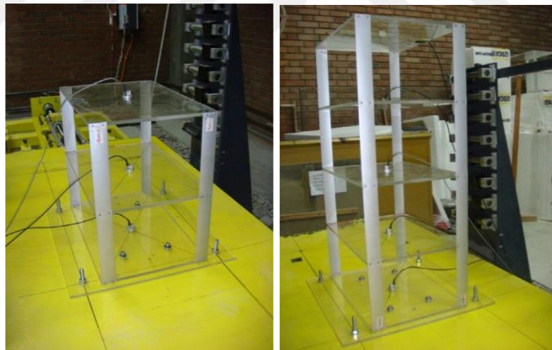
Figure 2.45. Three and Five Story Model Buildings (Kalpakci, 2013).
