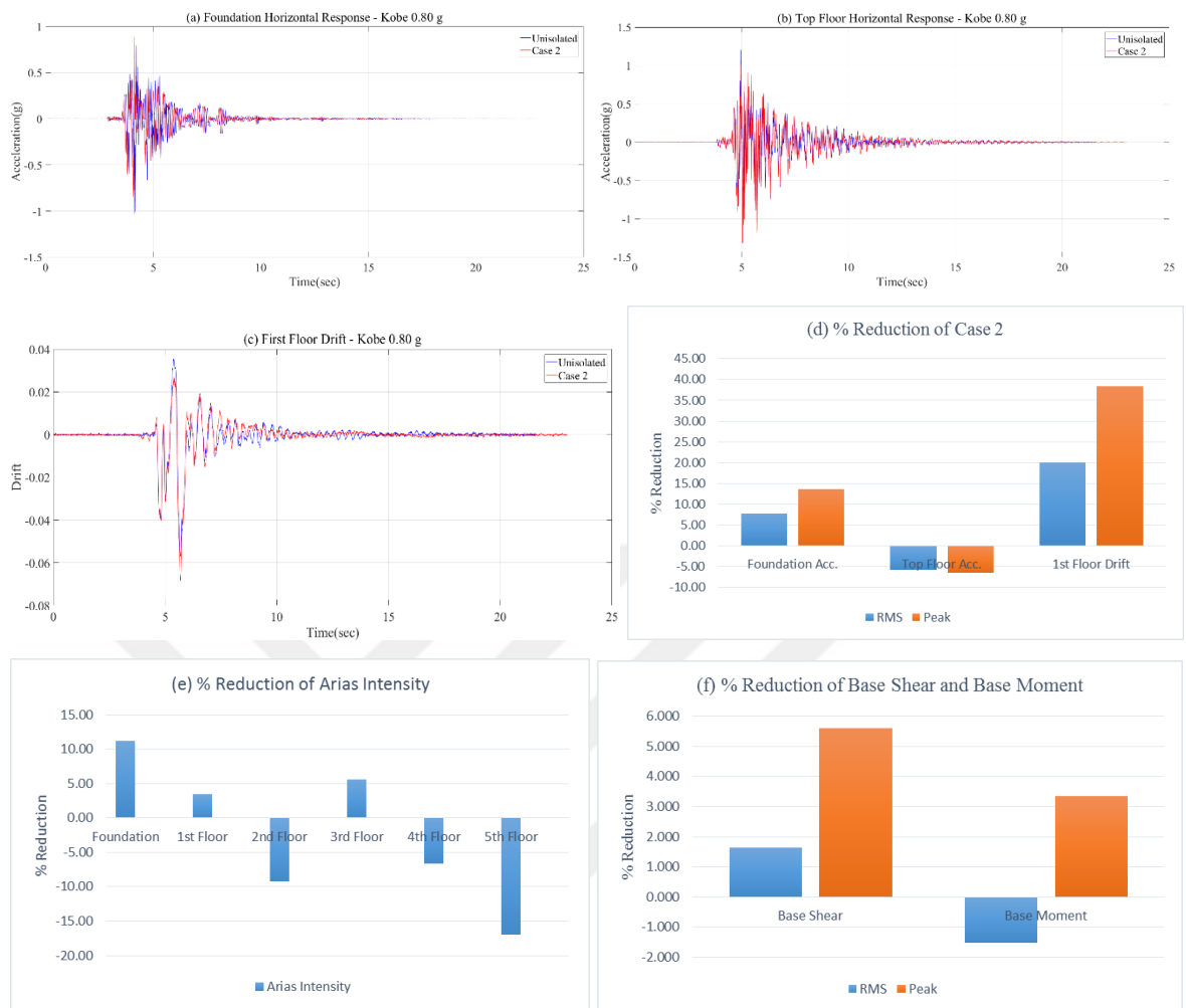
Figure 4.8. (a) Foundation Acceleration Response, (b) Top Floor Acceleration Response, (c) First Floor Drift Response, (d) % Reduction of Case 2, (e) % Reduction of Arias Intensity, (f) % Reduction of Base Shear and Base Moment under Kobe Earthquake.
