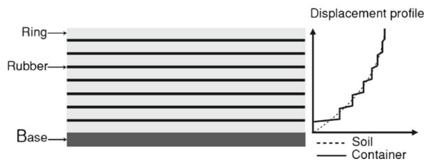
Figure 2.57. Schematic Demonstration of the Equivalent Shear Beam (Jafarzadeh, 2004).
