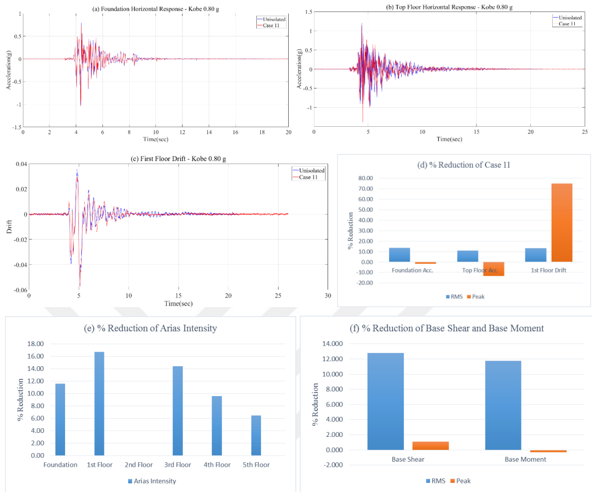
Figure 4.38. (a) Foundation Acceleration Response, (b) Top Floor Acceleration Response, (c) First Floor Drift Response, (d) % Reduction of Case 11, (e) % Reduction of Arias Intensity, (f) % Reduction of Base Shear and Base Moment under Kobe Earthquake.
