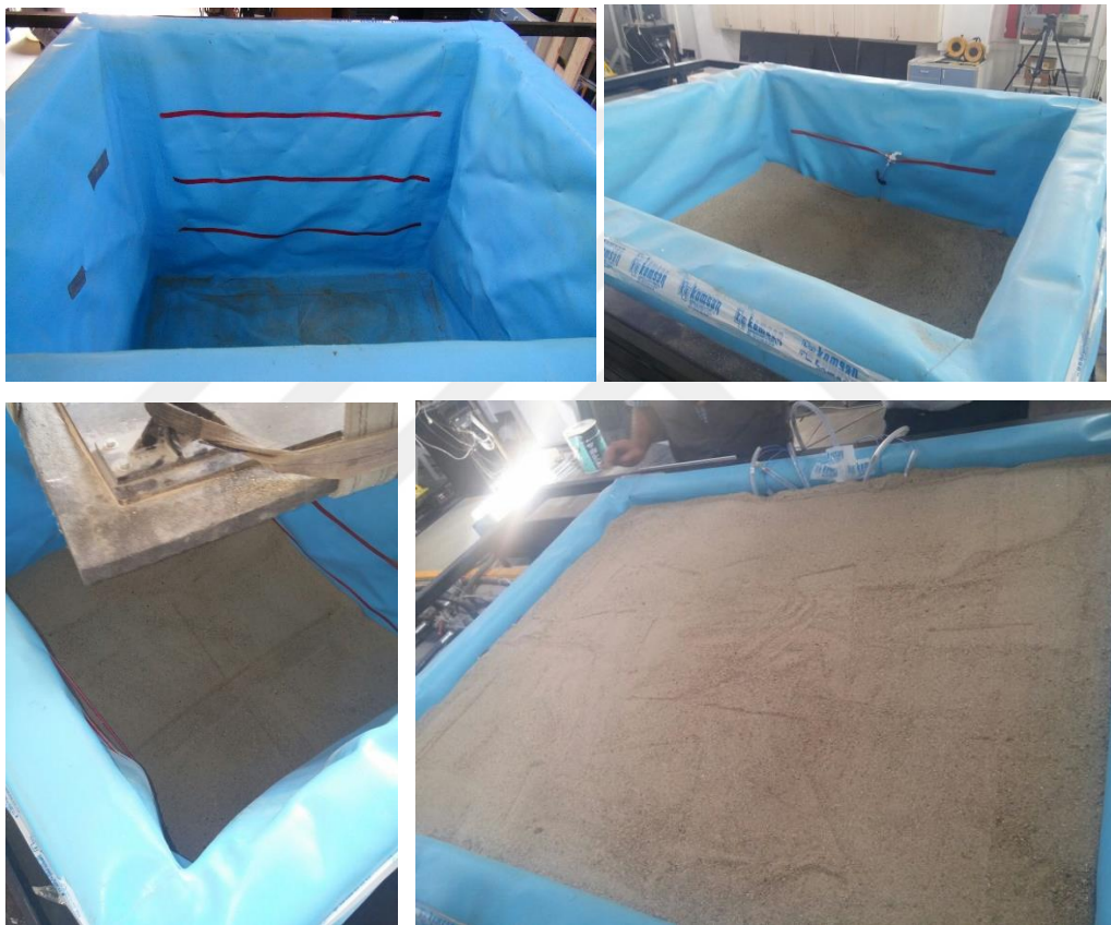
Figure 3.15. Soil Sample Preparation and Compaction.
