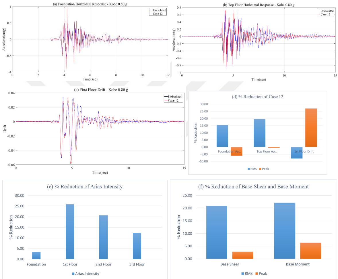
Figure 4.41. (a) Foundation Acceleration Response, (b) Top Floor Acceleration Response, (c) First Floor Drift Response, (d) % Reduction of Case 12, (e) % Reduction of Arias Intensity, (f) % Reduction of Base Shear and Base Moment under Kobe Earthquake.
