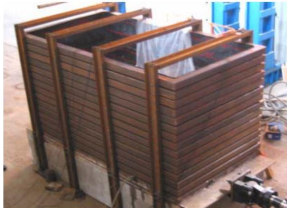
Figure 2.65. Empty Laminar Shear Box on the Shaking Table (Chunxia et al. , 2008).
