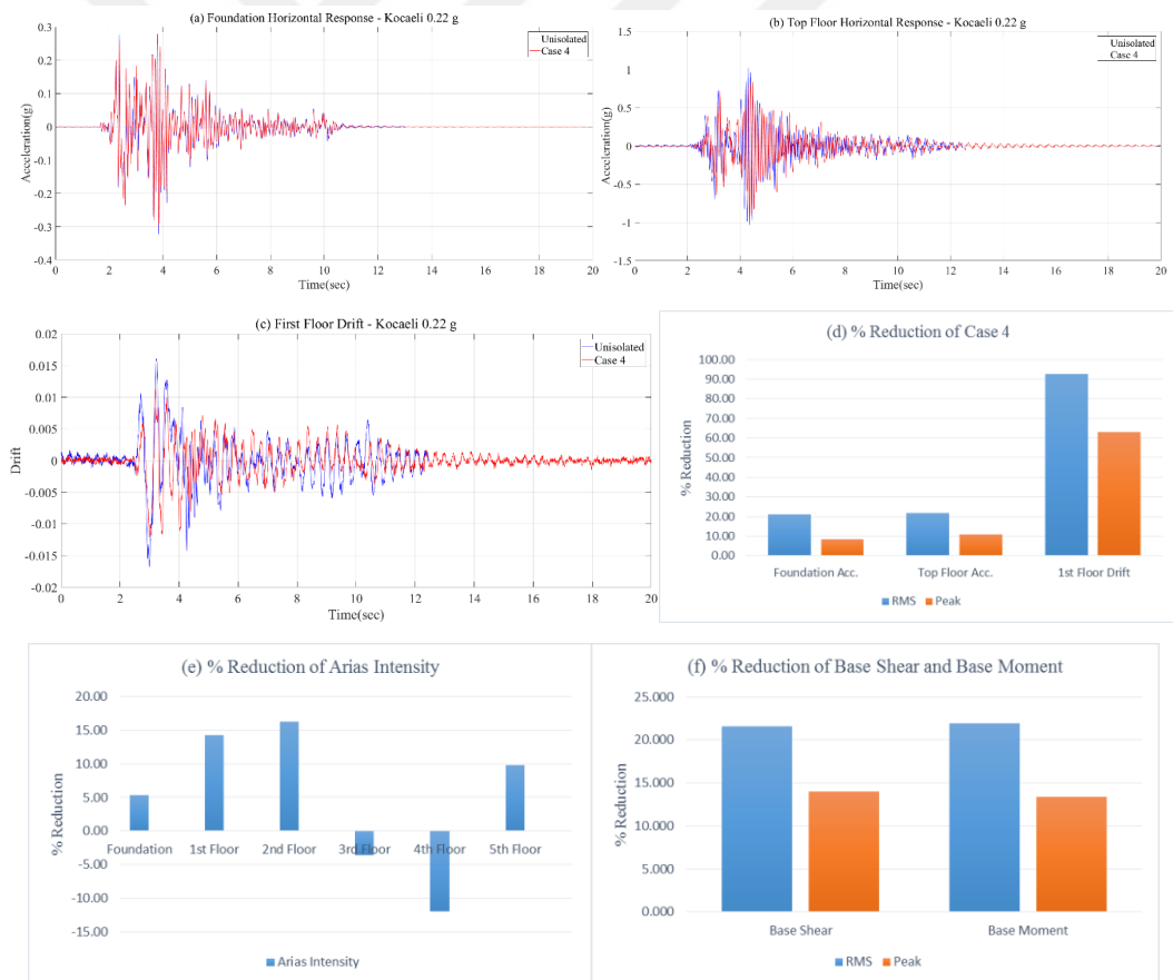
Figure 4.13. (a) Foundation Acceleration Response, (b) Top Floor Acceleration Response, (c) First Floor Drift Response, (d) % Reduction of Case 4, (e) % Reduction of Arias Intensity, (f) % Reduction of Base Shear and Base Moment under Kocaeli Earthquake.
