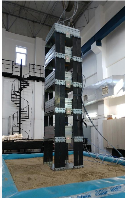
Figure 3.8. 1:10 Scaled Model of Five Story Building Model.
