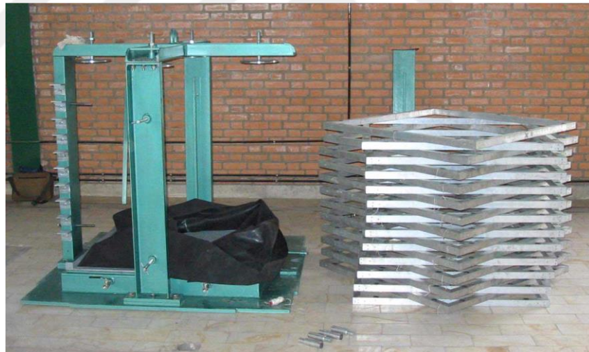
Figure 2.66. Disassembled Parts of A Laminar Box (Jafarzadeh, 2004).
