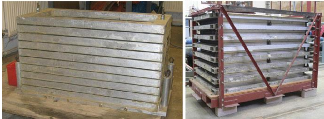
Figure 2.58. Examples of Equivalent Shear Beam Container (Jafarzadeh, 2004).
