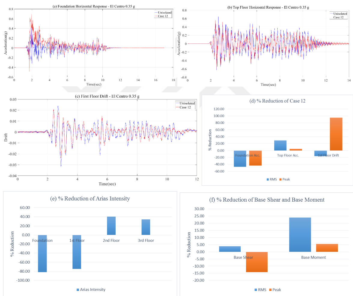
Figure 4.42. (a) Foundation Acceleration Response, (b) Top Floor Acceleration Response, (c) First Floor Drift Response, (d) % Reduction of Case 12, (e) % Reduction of Arias Intensity, (f) % Reduction of Base Shear and Base Moment under El Centro Earthquake.
