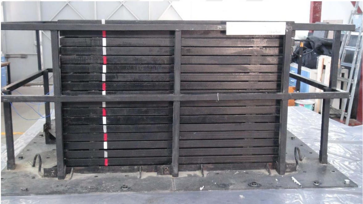
Figure 3.3. Side View of Unidirectional Laminar Box.
