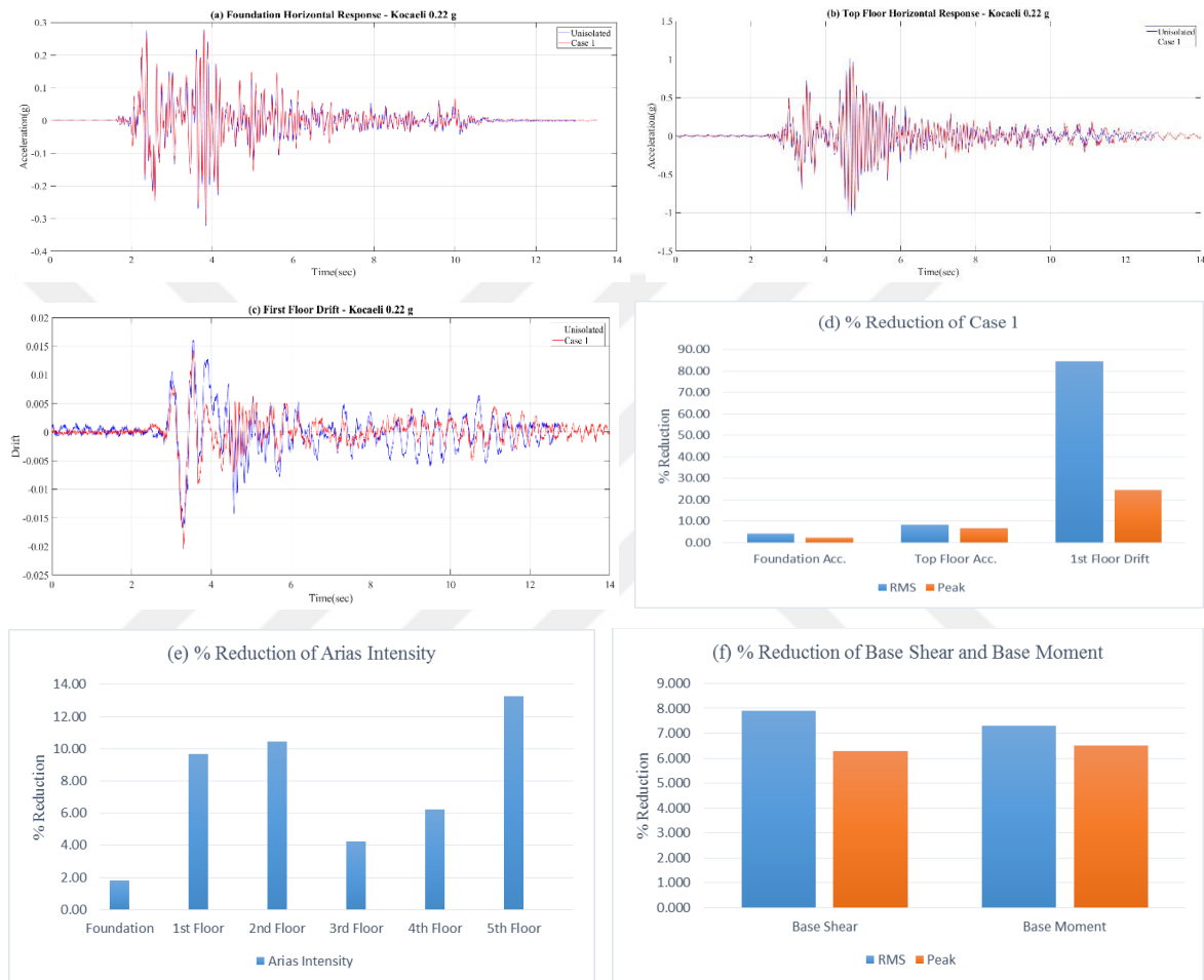
Figure 4.4. (a) Foundation Acceleration Response, (b) Top Floor Acceleration Response, (c) First Floor Drift Response, (d) % Reduction of Case 1, (e) % Reduction of Arias Intensity, (f) % Reduction of Base Shear and Base Moment under Kocaeli Earthquake.
