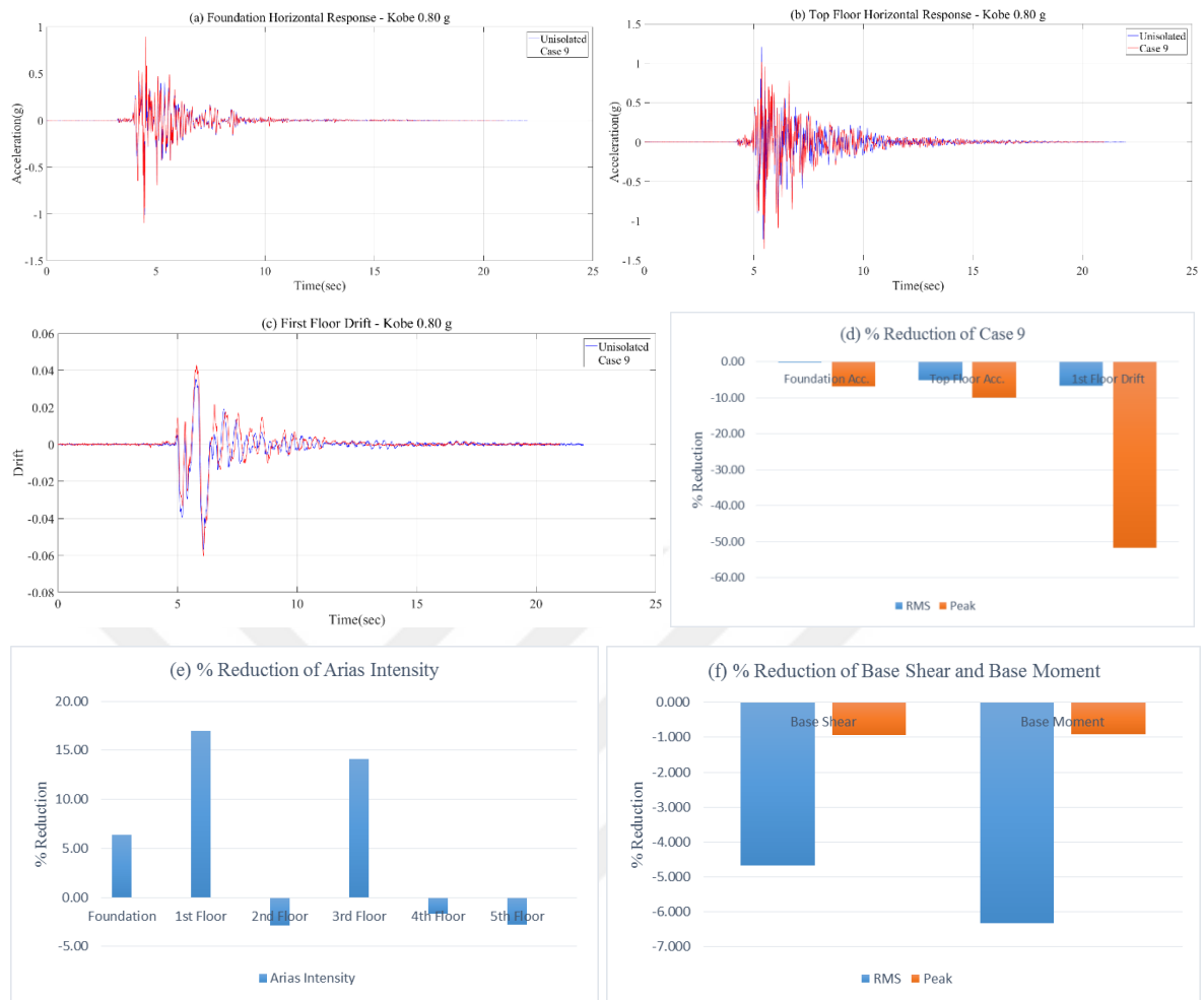
Figure 4.32. (a) Foundation Acceleration Response, (b) Top Floor Acceleration Response, (c) First Floor Drift Response, (d) % Reduction of Case 9, (e) % Reduction of Arias Intensity, (f) % Reduction of Base Shear and Base Moment under Kobe Earthquake.
