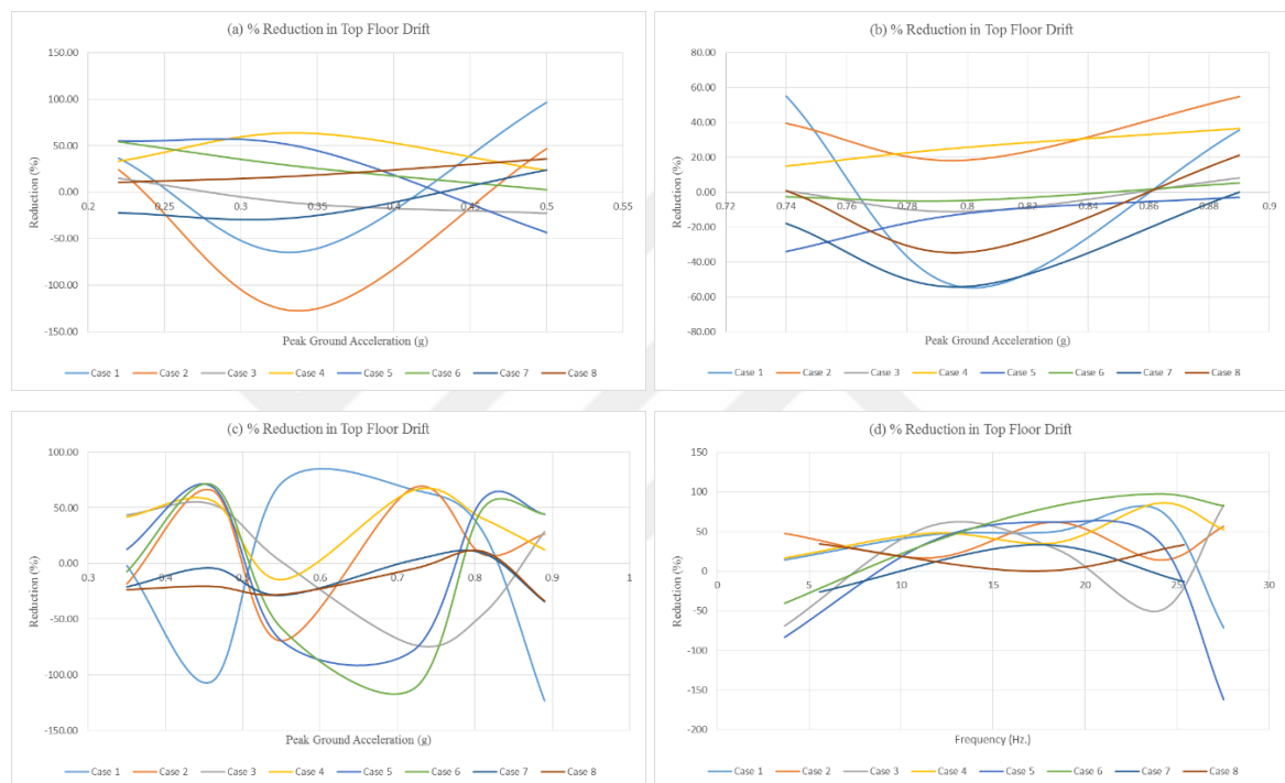
Figure 5.5. Reduction in Top Floor Drift under (a) Kocaeli Earthquake, (b) Kobe Earthquake, (c) El Centro Earthquake, (d) Cyclic Sinusoidal Motion for GSI-CL.
