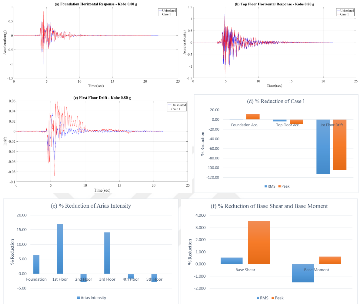
Figure 4.5. (a) Foundation Acceleration Response, (b) Top Floor Acceleration Response, (c) First Floor Drift Response, (d) % Reduction of Case 1, (e) % Reduction of Arias Intensity, (f) % Reduction of Base Shear and Base Moment under Kobe Earthquake.
