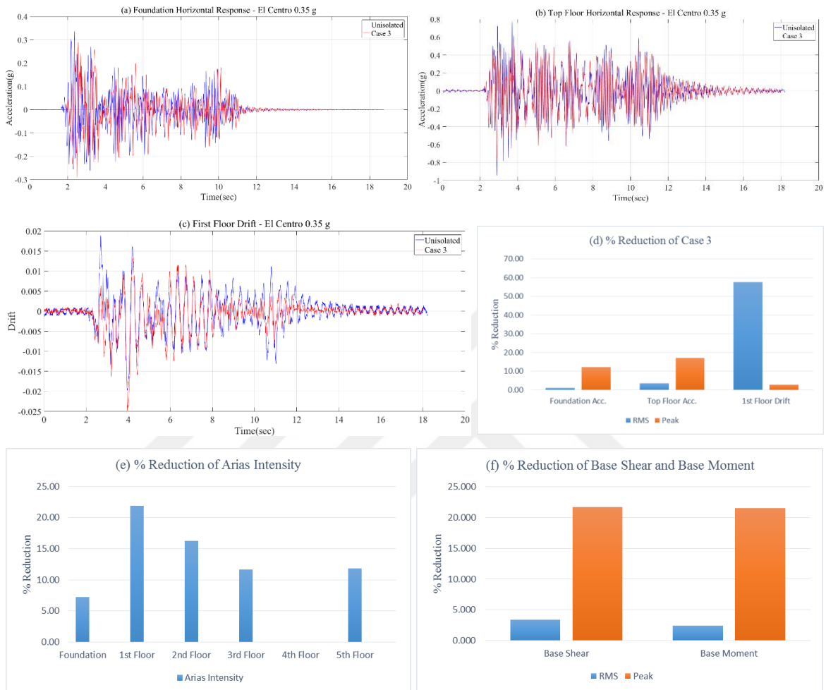
Figure 4.12. (a) Foundation Acceleration Response, (b) Top Floor Acceleration Response, (c) First Floor Drift Response, (d) % Reduction of Case 3, (e) % Reduction of Arias Intensity, (f) % Reduction of Base Shear and Base Moment under El Centro Earthquake.
