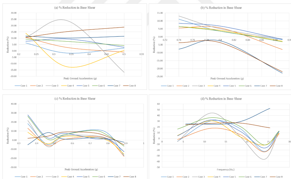
Figure 5.13. Reduction in Base Shear under (a) Kocaeli Earthquake, (b) Kobe Earthquake, (c) El Centro Earthquake, (d) Cyclic Sinusoidal Motion for GSI-CL.
