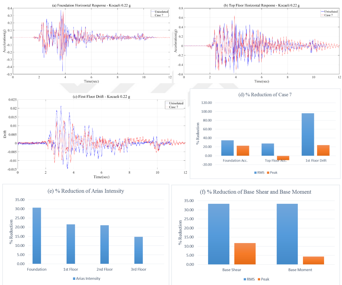
Figure 4.25. (a) Foundation Acceleration Response, (b) Top Floor Acceleration Response, (c) First Floor Drift Response, (d) % Reduction of Case 7, (e) % Reduction of Arias Intensity, (f) % Reduction of Base Shear and Base Moment under Kocaeli Earthquake.
