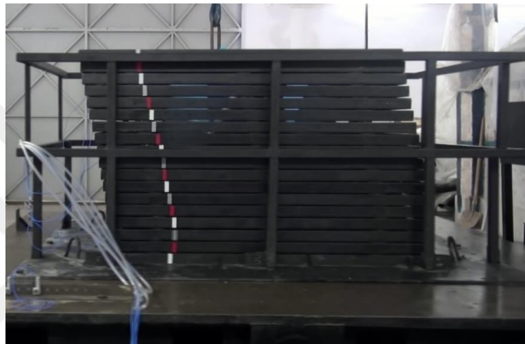
Figure 2.70. Side View of Unidirectional Laminar Box (Sekman, 2016; Goztepe, 2016).
