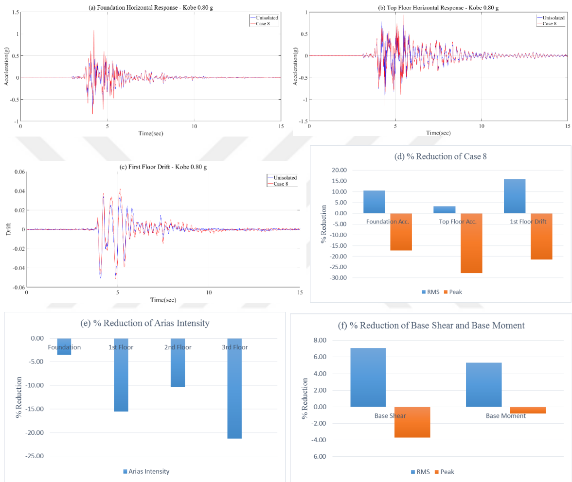
Figure 4.29. (a) Foundation Acceleration Response, (b) Top Floor Acceleration Response, (c) First Floor Drift Response, (d) % Reduction of Case 8, (e) % Reduction of Arias Intensity, (f) % Reduction of Base Shear and Base Moment under Kobe Earthquake.
