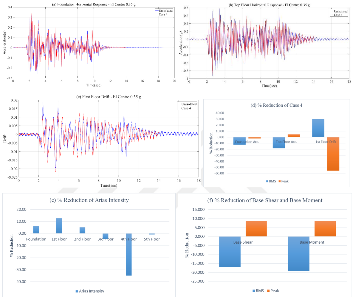
Figure 4.15. (a) Foundation Acceleration Response, (b) Top Floor Acceleration Response, (c) First Floor Drift Response, (d) % Reduction of Case 4, (e) % Reduction of Arias Intensity, (f) % Reduction of Base Shear and Base Moment under El Centro Earthquake.
