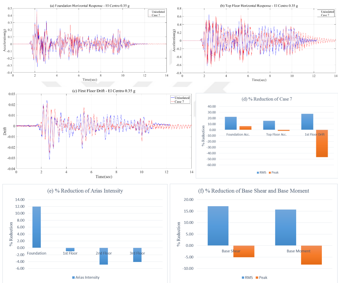
Figure 4.27. (a) Foundation Acceleration Response, (b) Top Floor Acceleration Response, (c) First Floor Drift Response, (d) % Reduction of Case 7, (e) % Reduction of Arias Intensity, (f) % Reduction of Base Shear and Base Moment under El Centro Earthquake.
