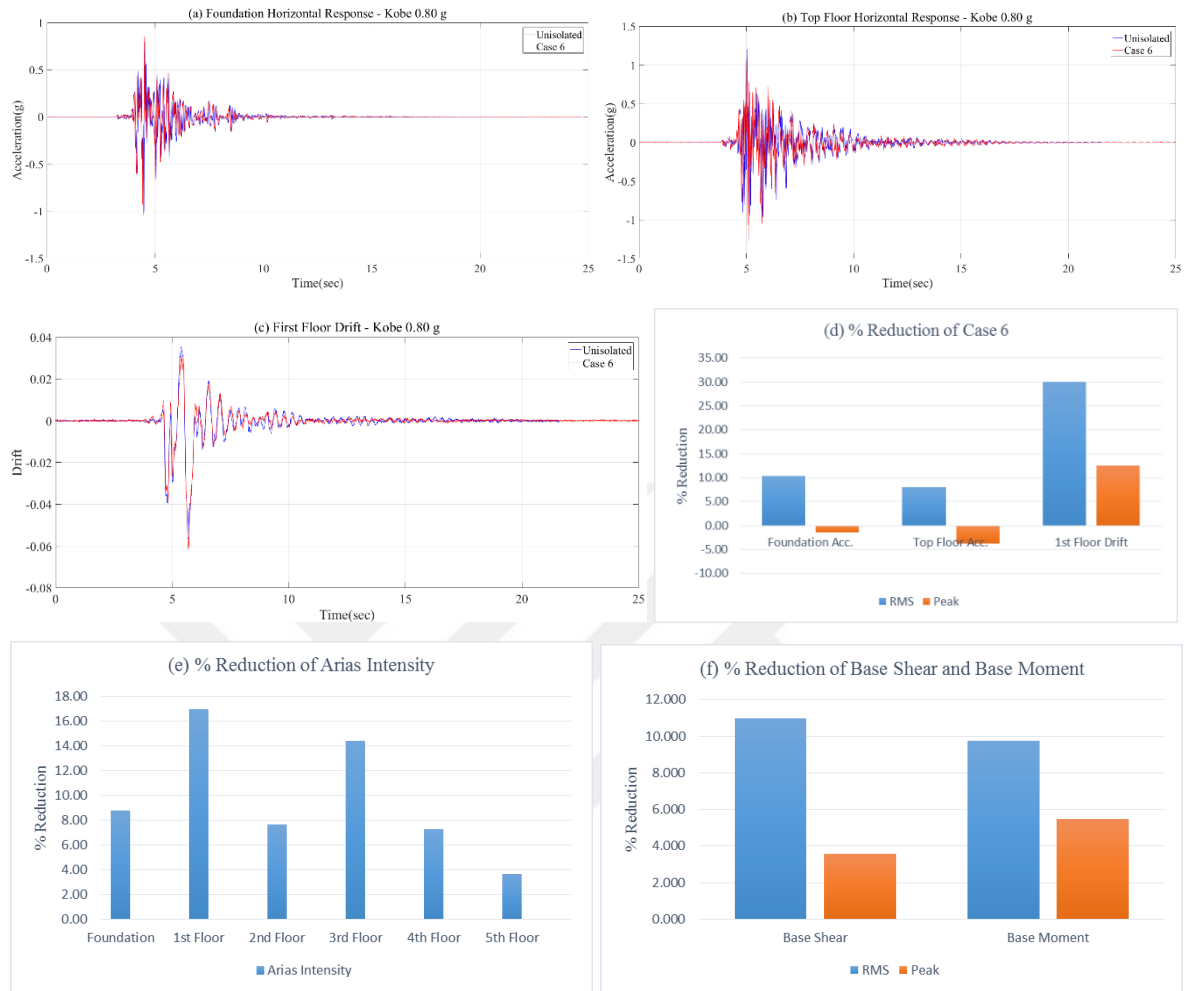
Figure 4.20. (a) Foundation Acceleration Response, (b) Top Floor Acceleration Response, (c) First Floor Drift Response, (d) % Reduction of Case 6, (e) % Reduction of Arias Intensity, (f) % Reduction of Base Shear and Base Moment under Kobe Earthquake.
