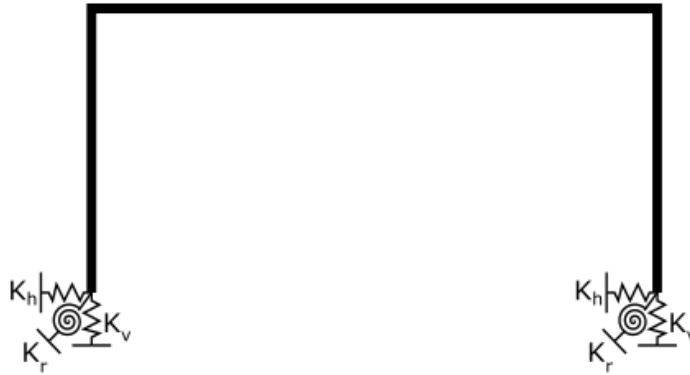
Figure 6.3. Representation of soil-structure system.
