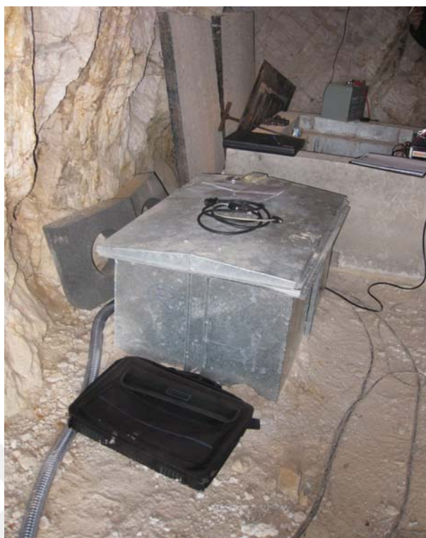
Figure B4. Photo of the second housings next to the two of the PIRES Arrays stations (POWD and FUTB) on Sivriada and Yassiada Islands.
