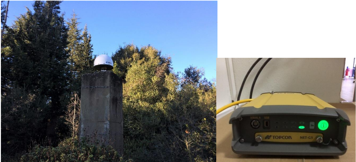
Figure 1.1. GPS receiver named KANT functioning 24 hours/day (Trimble NETR9, now TOPCON Net-G5 with a choke-ring model antenna).
