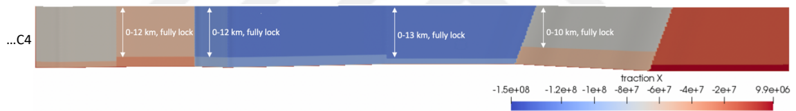
Figure 5.11. Initial shear (along strike) tractions on the fault surface for a fully locked model; ‘...C4’.
