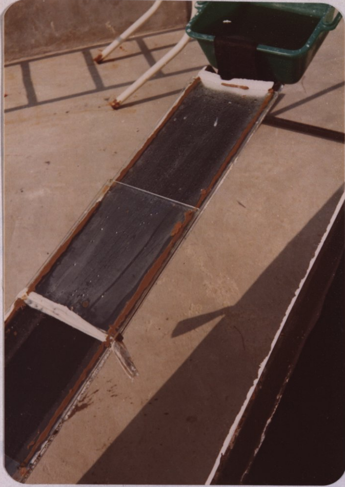
CONDENSATION PROBLEM IN LONG CHANNEL TYPE EVAPORATORS
