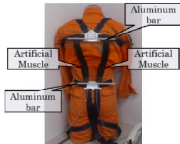
Fig. 4. Power assist suit with two artificial muscles
