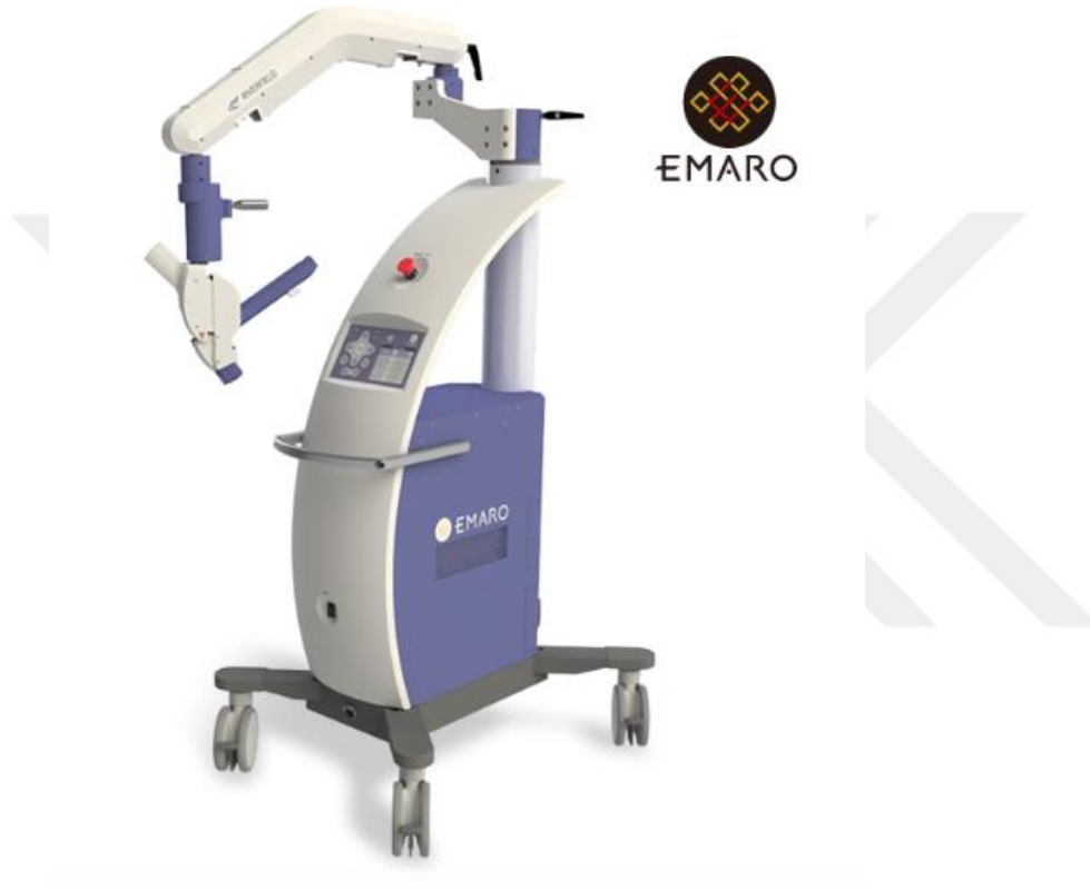
Figure 17. Riverfield’s robotic surgeon Emaro Source: Riverfield Inc, 空気圧駆動型 内視鏡ホルダロボット EMARO Kūkiatsu kudō-gata naishikyō horudarobotto [EMARO Pneumatic Endoscope Manipulator Robot]
