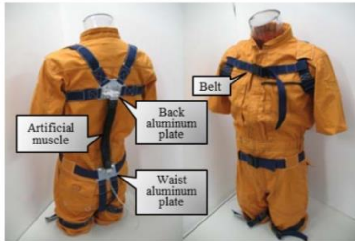
Fig. 3. Power assist suit with one artificial muscle
