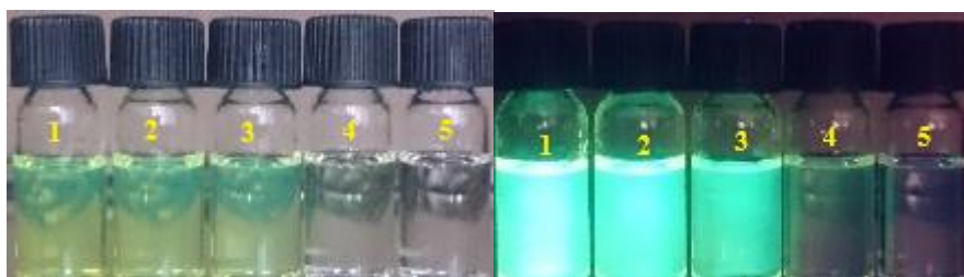
Figure 4.26. Left: Color change under Ambient light for the titration of a mixture containing 27 (10 \mu\text{M} ) in DMSO and TBAOH (0-5 equiv.) in DMSO, with the incremental addition of TFA (0-5 equiv) in DMSO solution; Right: Color change under 365 nm UV light for the titration of a mixture containing 3g (10 \mu\text{M} ) and TBAOH (0-5 equiv.) in DMSO, with the incremental addition of TFA (0-5 equiv) in DMSO solution. Description; 1: Host + TBAOH (5 equiv) + TFA (1 equiv); 2: Host + TBAOH (5 equiv) + TFA (2 equiv); 3: Host + TBAOH (5 equiv) + TFA (3 equiv); 4: Host + TBAOH (5 equiv) + TFA (4 equiv); 5: Host + TBAOH (5 equiv) + TFA (5 equiv)
