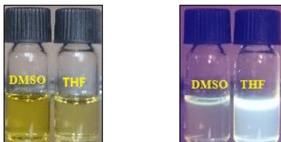
Color changes of 31 under Ambient light Color changes of 31 under 365 nm UV light
