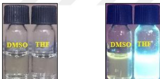
Color changes of 35 under Ambient light Color changes of 35 under 365 nm UV light
