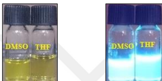
Color changes of 34 under Ambient light Color changes of 34 under 365 nm UV light
