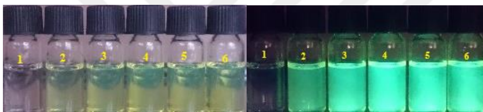
Figure 4.25. Left: Color change under Ambient light for the titration of 27 (10 \mu\text{M} ) in DMSO with incremental addition of TBAOH (0-5 equiv) in DMSO solution; Right: Color change under 365 nm UV light for the titration of 27 (10 \mu\text{M} ) with incremental addition of TBAOH (0-5 equiv) in DMSO solution. Description; 1: Host; 2: Host + TBAOH (1 equiv); 3: Host + TBAOH (2 equiv); 4: Host + TBAOH (3 equiv); 5: Host + TBAOH (4 equiv); 6: Host + TBAOH (5 equiv)
