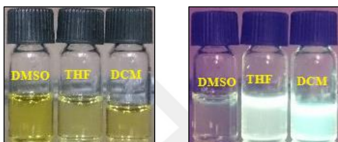
Color changes of 30 under Ambient light Color changes of 30 under 365 nm UV light
