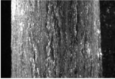
Head: 153 m Model Nozzle opening: 80% Jet diameter: 34mm
