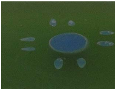
Figure 6.12. MR LOCL LC cement surface (a) at the beginning (b) after 7 day immersion in (pH 4.0)
