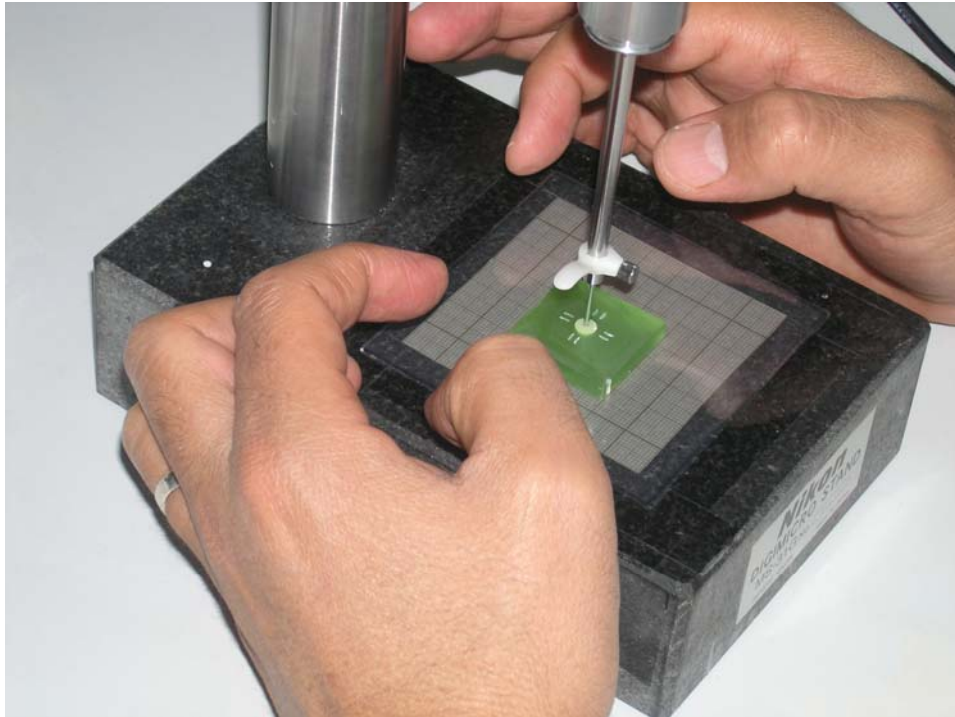
Figure 5.13 Depth loss measuring
