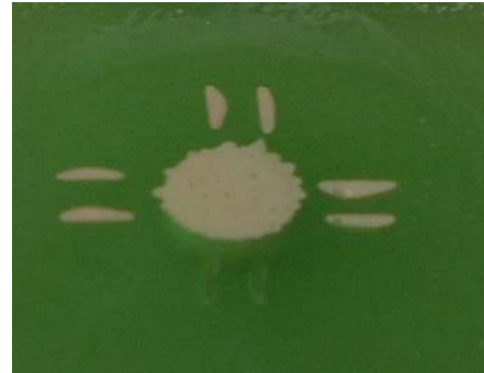
Figure 6.9 Ultra Band LoK cement surface (a) at the beginning (b) after 7 day immersion in (pH 2.74)
