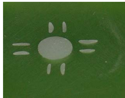
Figure 6. 14 Multi cure Glass ionomer cement surface (a) at the beginning (b) after 7 day immersion in (pH 4.0)
