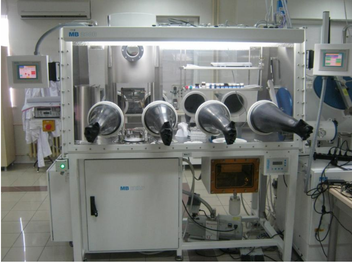
ekil 3.1: Termal evapulator (Leybold PVD systems) cihazı
