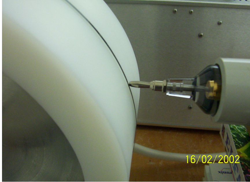
Şekil 3.3. Tektronix P6015A 1000x3,0 pF 100 MΩ Prop
