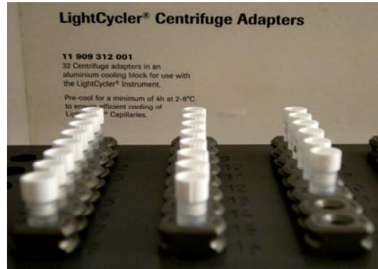
Resim13: Kapiller adaptör (LightCycler ® Centrifuge Adapters).
