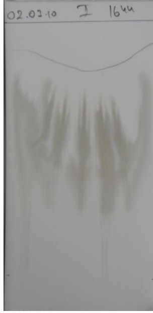
Şekil III.7. Mobil Faz: Toluen: Metanol: Formik asit (30:32:8). Örnek konsantrasyonları: EA6: 4.9 \times 10^{-3} mol.L -1 EA8: 5.8 \times 10^{-3} mol.L -1 EA9: 6.0 \times 10^{-3} mol.L -1 EA10: 8.3 \times 10^{-3} mol.L -1 EA11: 8.7 \times 10^{-3} mol.L -1 .
