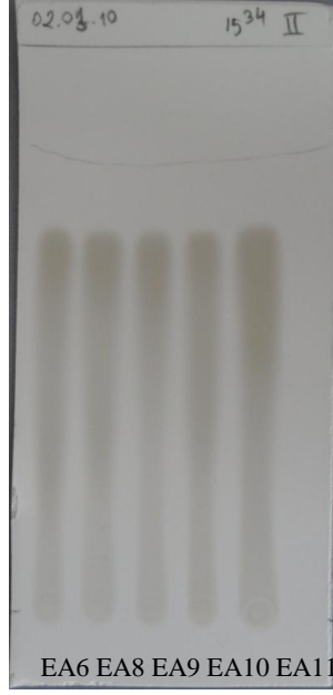
Şekil III.8. Mobil Faz: Toluen: Aseton: Formik asit: Metanol (30:30:8:2). Örnek konsantrasyonları: EA6: 4.9 \times 10^{-3} mol.L -1 EA8: 5.8 \times 10^{-3} mol.L -1 EA9: 6.0 \times 10^{-3} mol.L -1 EA10: 8.3 \times 10^{-3} mol.L -1 EA11: 8.7 \times 10^{-3} mol.L -1 .
