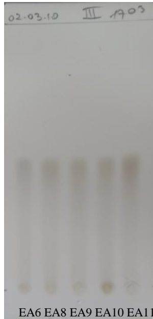
Şekil III.1. Mobil Faz: Toluen: Etil Asetat: Formik asit: Metanol (30:30:8:2). Örnek konsantrasyonları: EA6: 4.9 \times 10^{-3} \text{ mol.L}^{-1} EA8: 5.8 \times 10^{-3} \text{ mol.L}^{-1} EA9: 6.0 \times 10^{-3} \text{ mol.L}^{-1} EA10: 8.3 \times 10^{-3} \text{ mol.L}^{-1} EA11: 8.7 \times 10^{-3} \text{ mol.L}^{-1} .
