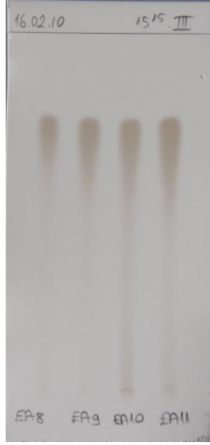
Şekil III.9. Mobil Faz: Toluen: THF: Formik asit: Metanol (30:30:8:2). Örnek konsantrasyonları: EA8: 5.8 \times 10^{-3} mol.L -1 EA9: 6.0 \times 10^{-3} mol.L -1 EA10: 8.3 \times 10^{-3} mol.L -1 EA11: 8.7 \times 10^{-3} mol.L -1 .
