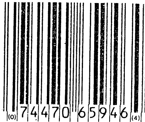
Figure 2.3 An example of product coding. Bars and spaces may have four different widths. Two bars and two spaces make up a single digit.
