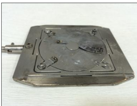
Figure 4.5: Pt(111) single crystal mounted on a holder.
