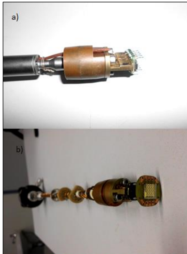
Figure 3.9: Sample holder with special chip carrier. a) Front end of the cryostat insert with the ten-pins connector. b) Complete cryostat insert with a sample holder plugged into the connector. The bonding wires between the electrodes of the sample and the pads of sample holder can hardly be seen.
