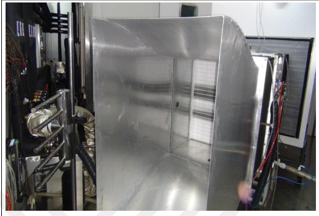
Figure 5.7: The evaporator under frosting test at conditioning room.
