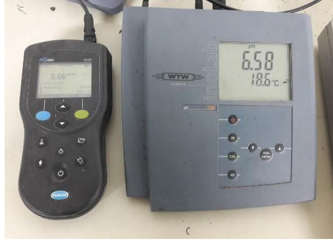
WTW multi340i (solda) ve Inolab WTW-ph720 (sağda)
