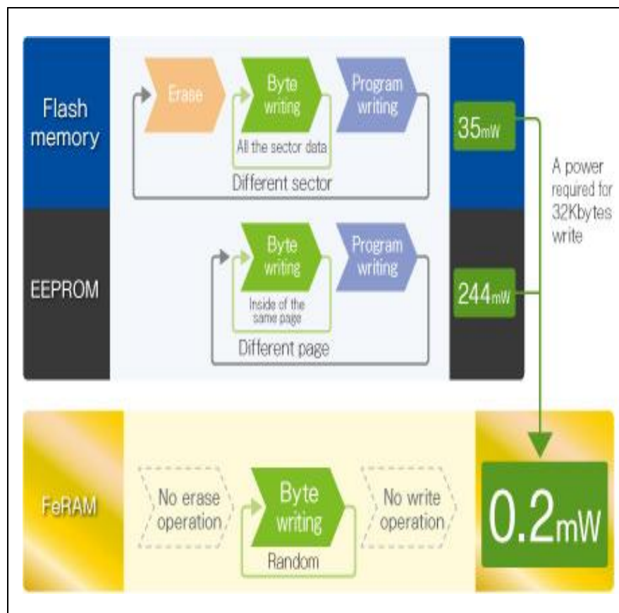
Figure 2.3: There are no mechanisms of erasing and writing operations. Byte writing speed is fast even power down in FeRAM.
