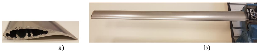
Figure 1.1: Photos of elastic blade structure a) cross-section view, b) longitudinal view.
