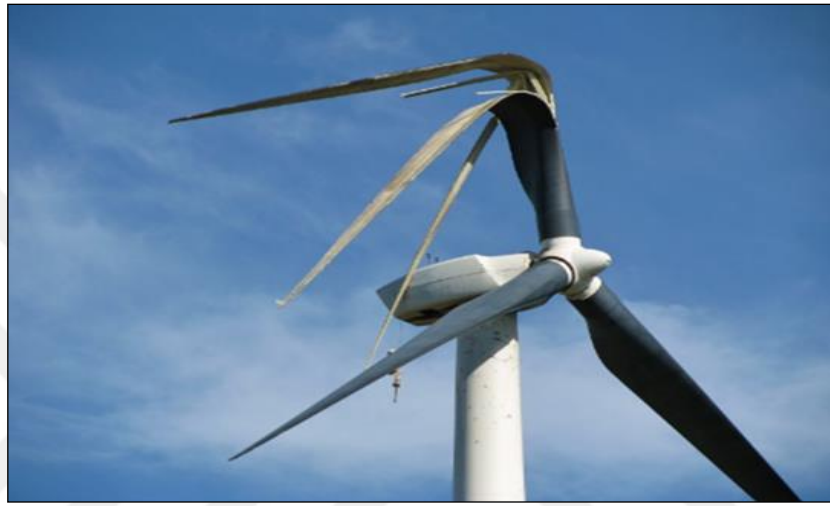
Figure 1.2: A damaged wind blade due to vibration.
