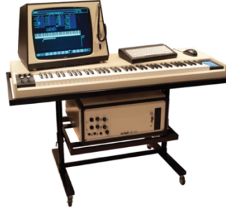
Şekil 2. 46: The Fairlight CMI (Computer Music Instrument) Digital Synthesizer (Vintage: Fairlight CMI Series.,2016).
