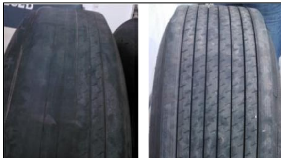
Figure 1.1: Tire wear, a) partial abrasion, b) normal state [Du et al., 2017].
