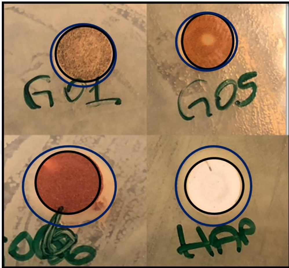
Figure 3.19: Antibacterial test results of 0,0010 (GO1) and 0,0020 (GO5) and 0,0030 (GO6) mole Zn-Fe co-doped HAP pellets respectively.
