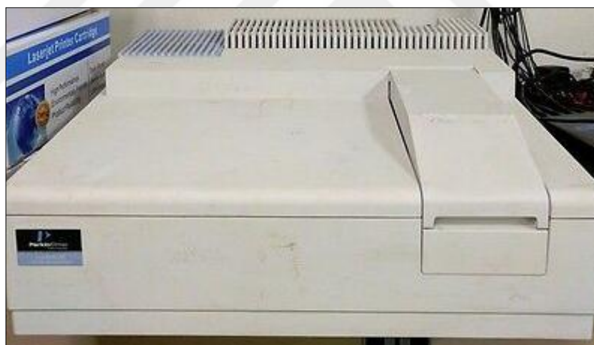
Figure 3.10: Perkin Elmer Lambda 35 UV/vis Spectrometer.
