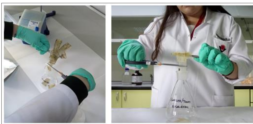
Figure 2.9: SPMDs are cutting into little pieces.
