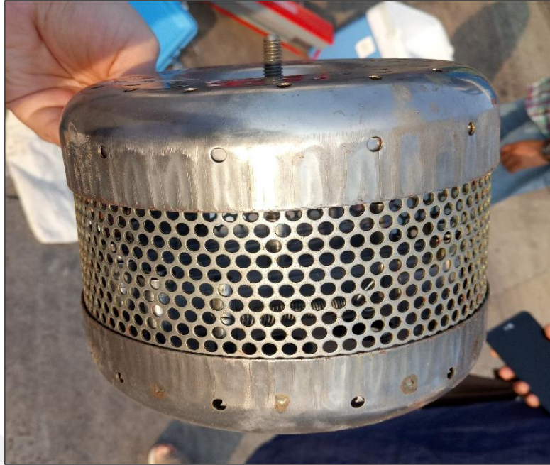
Figure 1.3: SPMDs in steel cage.
