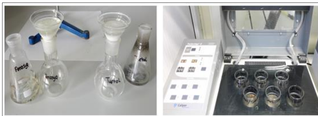
Figure 2.11: Sodium Sulphate column and volume decreasing at Zaymark Turbovaps.
