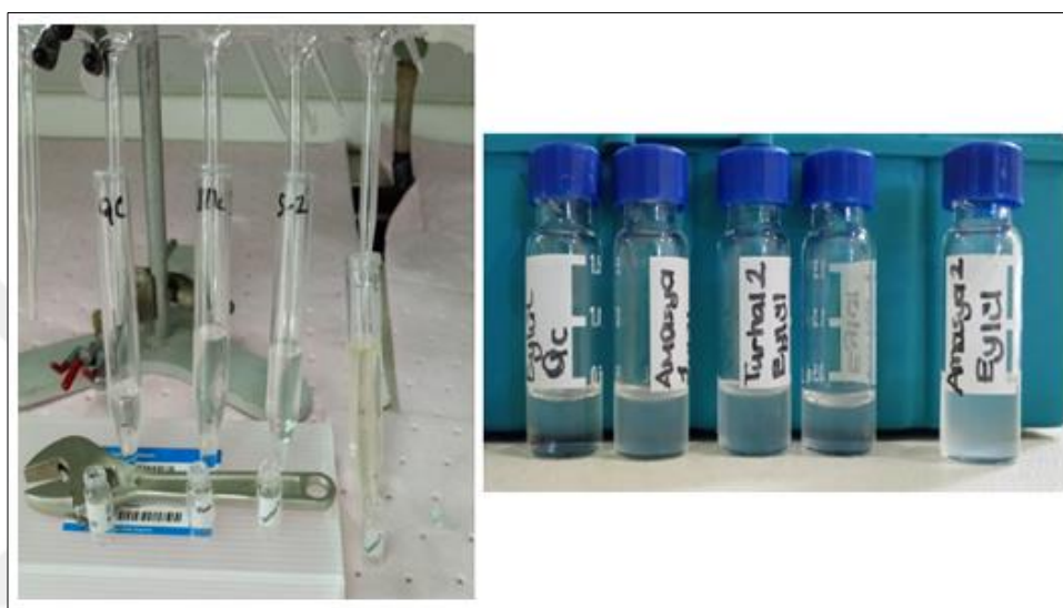
Figure 2.14: Volume decreasing of the sample and take it to the vials.
