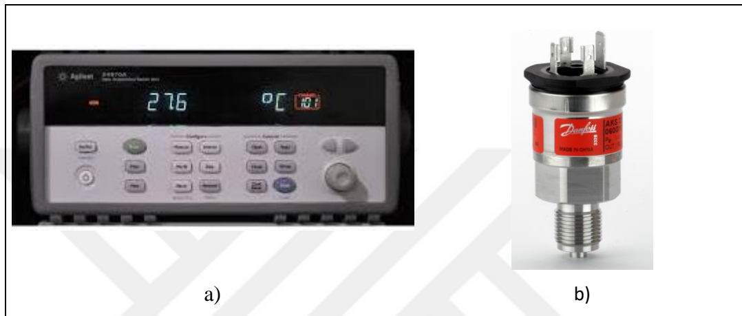
Figure 4.6: a) Agilent 34970A data logger, b) Danfoss AKS 32R pressure transducer.
