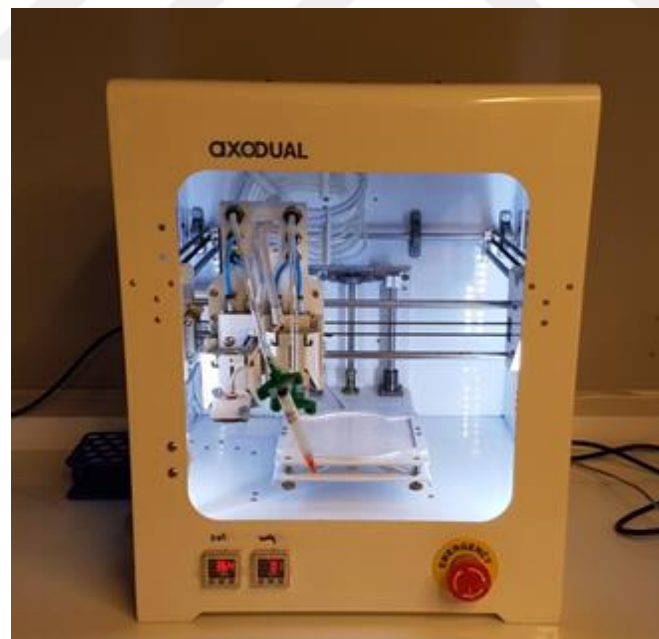
Figure 3.3: The syringe with orange head loaded bio-printer.
