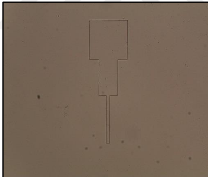
Figure 4.11: Photomicrograph of the gate metal (the image was taken after M1 deposition and deposition of \text{SiN}_x/\text{Al}_2\text{O}_3 -bilayer gate dielectric-, and amorphous silicon layers).
