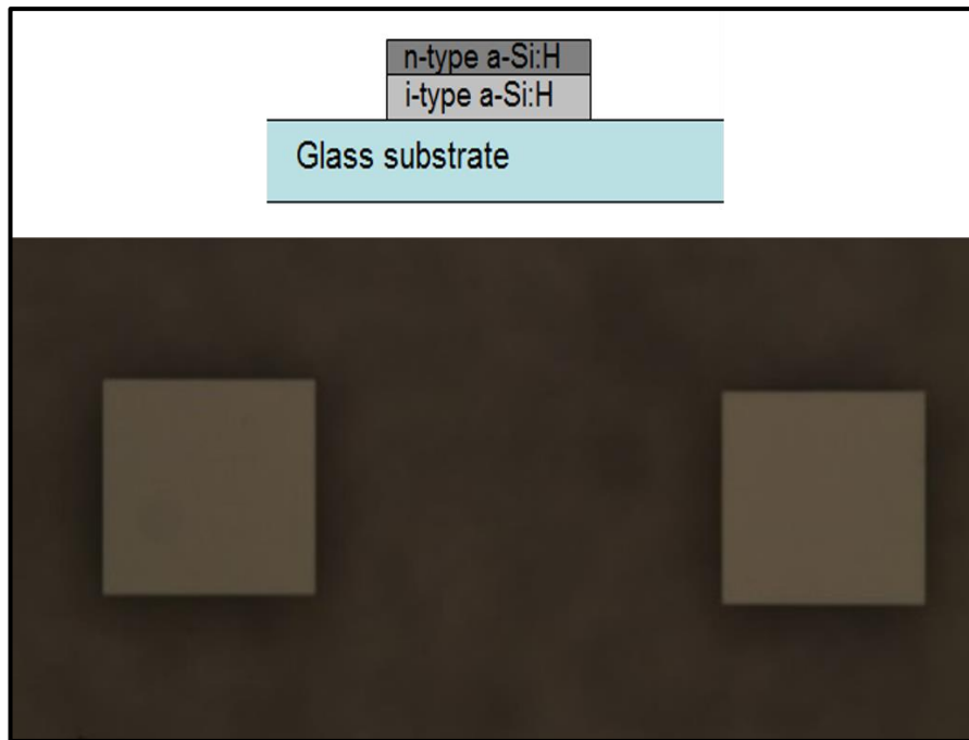
Figure 4.4: Schematic cross-sectional view and photomicrograph of the island (active device area).
