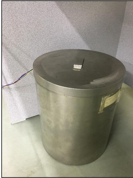
Figure 5.13: Three-layered mu-metal shielding.
