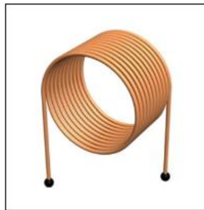
Figure 3.2: The simplest induction sensor.
