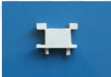
Figure 5.8: One of the plate produced for pick-up coil windings.
