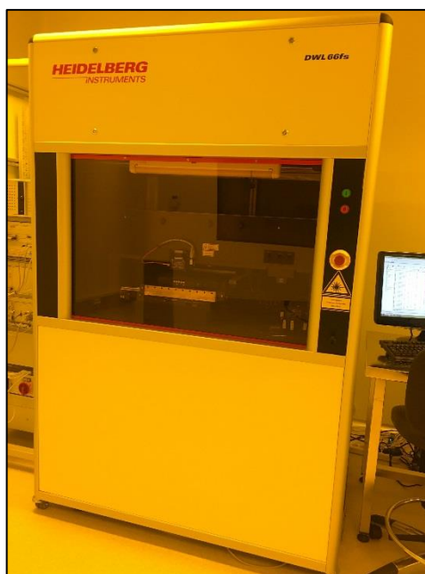
Figure 5.2: Mask printer device at Gebze Technical University, Nanotechnology Institute, Clean Room Laboratory.
