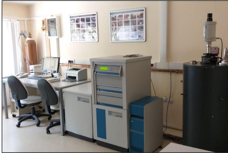
Figure 5.1: Vibrating sample magnetometer at Gebze Technical University, Physics Department, Physical Property Measurement System (PPMS) Laboratory.
