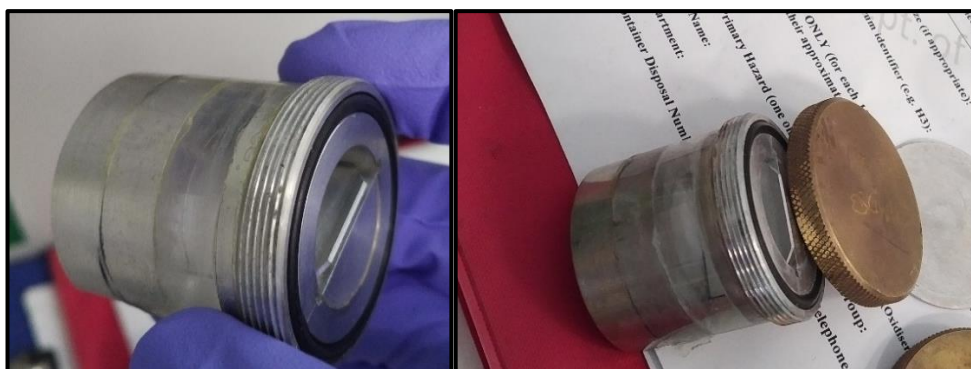
Figure 2.6: Air tight sample holder for XRD analysis.
